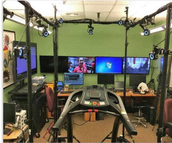
Figure 1: Setup for the movement data collection. The treadmill was surrounded by a motion tracking system, for which the approximate capture area was limited to the head of each subject. Cameras were calibrated before each session.
