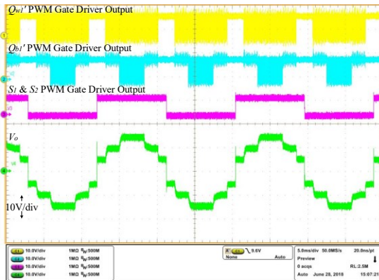
(e) Tested output voltage in relation to PWM signals of two switched capacitor cells and the full-bridge unfolded ( V_{in} = 5V )
