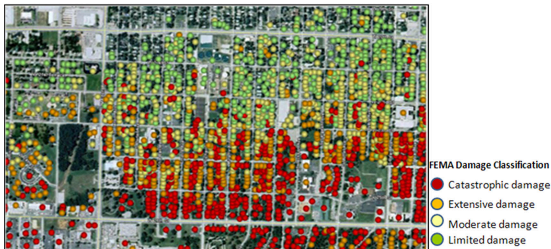
FIGURE 9 | Per-building analysis of damaged buildings in Joplin, MO (2011). Image Credit: ImageCat (used with permission).
