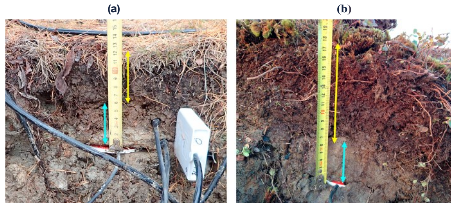
Figure E1. An example of installation of heat flux plate at the depth of 6 cm (cyan arrow) below the top of mineral soil in the Polar Urals, Russia. (a) The thickness of the "O" horizon and peat layer (yellow arrow) containing undecomposed and partially decomposed organics is ~6 cm. (b) For a different site with the same instrumentation setup, the peat thickness is ~12 cm, also containing a surface moss layer. Soil temperature sensors at the depths of 2 and 4 cm (black cables) as well as averaging soil moisture and temperature sensor at the same depth range (white plastic head) can be seen to the right of the heat flux plate in (a).
