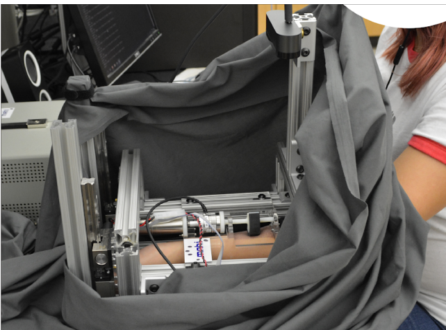
Fig. 7. Device in use during validation experiment. Note that subject's view of the device was obstructed and the subject listened to pink noise to prevent them from hearing the actuation of the motors.
