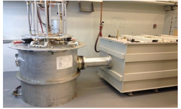
Fig. 2. The 500 kV, 200 A electron gun connected to a 500 kV, 250 A Marx modulator in the Beam Physics Lab at Yale University.
