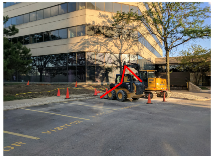
Fig. 15. False prediction result of the bucket due to occlusion.
