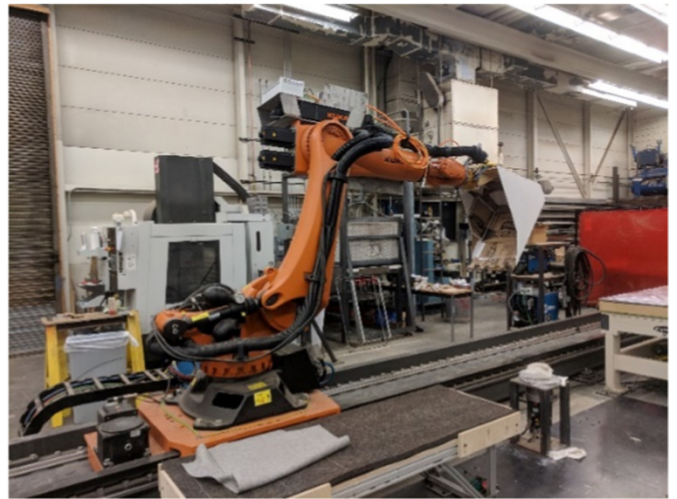
Fig. 7. The simulated robotic excavator - robot arm mounted with an excavator bucket.
