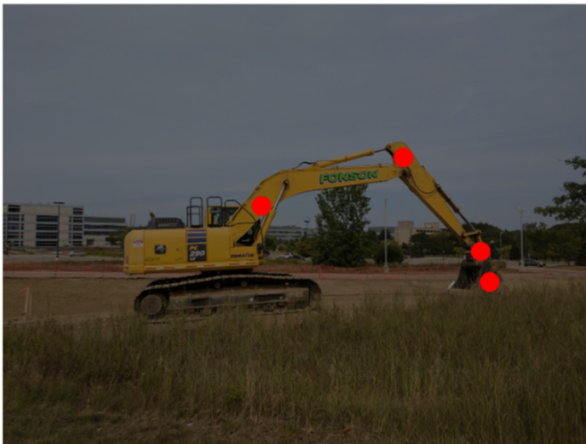
Fig. 5. The concept of the prediction heat-map generated by the output prediction module. Each circle represents the highest probability of corresponding joint location.
