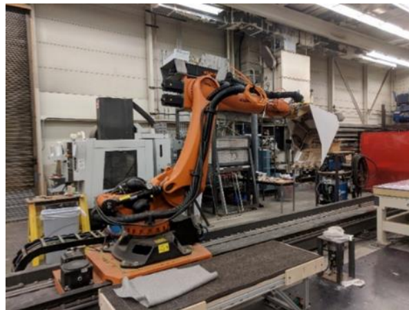
Figure 2. The simulated robotic excavator - robot arm mounted with an excavator bucket.
