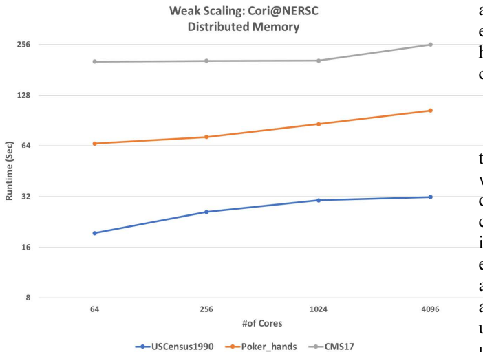
Fig. 6. Weak scaling of adaptive anonymity algorithm on Cori.
