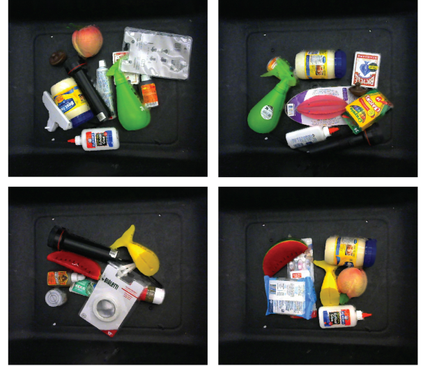
Fig. 4: Example bins from the WISDOM-Real test set. The number of objects in each bin was chosen from a Poisson distribution with mean 5, with a minimum of two objects per bin. The highly-varied geometry and occlusions make these bins challenging to segment.
