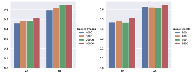
Fig. 6: Effect of increasing synthetic training dataset size (left) and increasing the number of unique objects (right) on the performance of SD Mask R-CNN on the WISDOM-Real high-res test set. These results suggest that more data could continue to increase performance.
