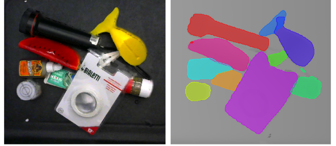
Fig. 1: Color image (left) and depth image segmented by SD Mask RCNN (right) for a heap of objects. Despite clutter, occlusions, and complex geometries, SD Mask RCNN is able to correctly mask each of the objects.
