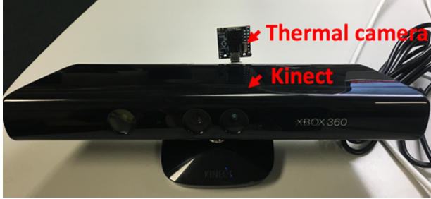
Fig. 2. The dual camera system (thermal camera coupled with Microsoft Kinect).
