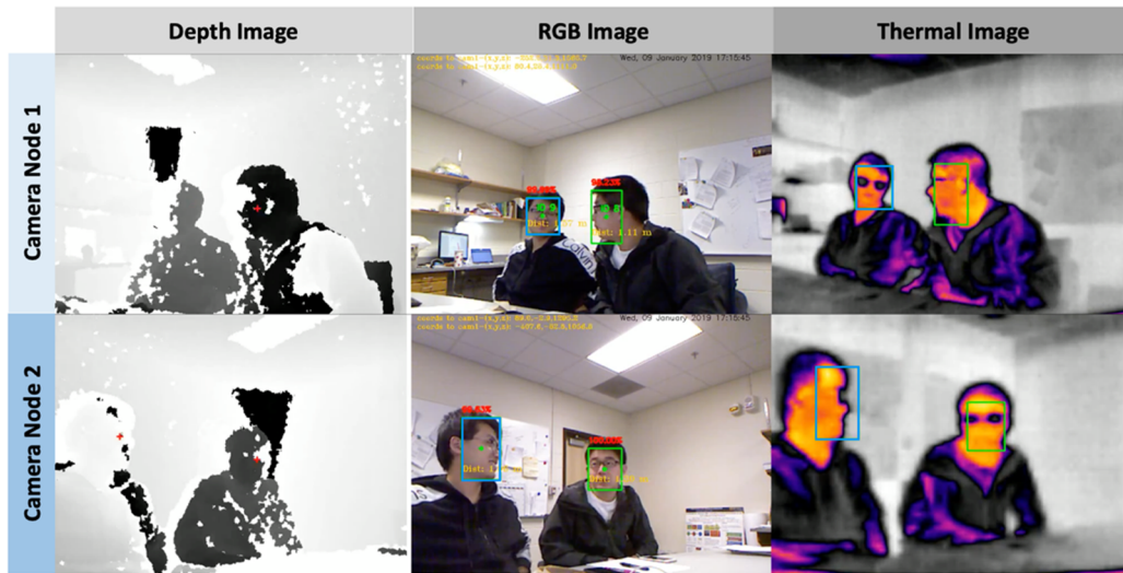
Fig. 12. Image frames collected in the experiment (row 1: views from camera node 1; row 2: views from camera node 2).
