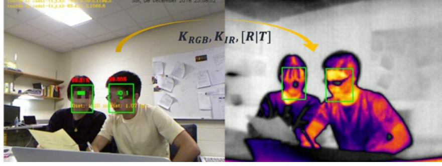
Figure 4: Dual Camera Face Detection. Left: RGB Images from the Kinect (for Face Detection); Right: Thermal Images from the Thermographic Camera (bounding boxes are mapped from the RGB image)
