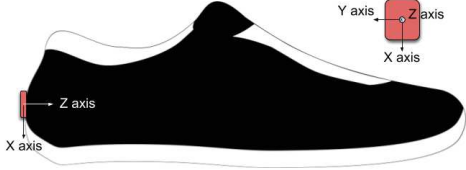
Fig. 1: Sensor placement and axis orientation.
