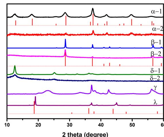
**Figure 1.** XRD patterns of different MnO<sub>2</sub> structures. The vertical lines are the corresponding standard patterns for the MnO<sub>2</sub> in the inorganic crystallographic database.
