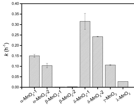
**Figure 2.** Pseudo-first-order oxidation rate constants ( $k$ ) of BPA by different  $\text{MnO}_2$  structures at pH 5. Error bars are the standard deviation of duplicate samples. Conditions:  $[\text{MnO}_2]$  138  $\mu\text{M}$ ; BPA 6  $\mu\text{M}$ ; [NaCl] 0.01 M.
