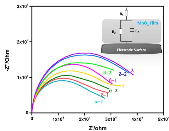
**Figure 3.** Nyquist plots obtained from EIS measurements of the  $\text{MnO}_2$ . Inset: equivalent circuit used to obtain charge-transfer resistance of different structured  $\text{MnO}_2$ .
