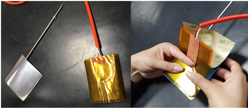
Fig. 12. Views of the aluminum wing and heating film on the top surface of the wing.
