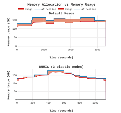
(c) between Memory allocation and Memory usage on default mesos and RUMIG with 3 elastic nodes.
