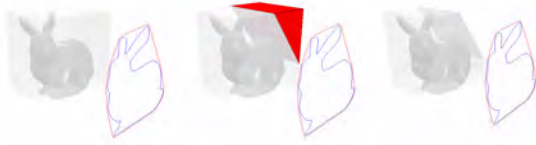
Figure 8: Planar cuts are generated from the convex hull of the silhouette. (a) Silhouette in a specific direction. (b) The red region represents the material to be removed by a planar cut. (c) The model after removing the material.
