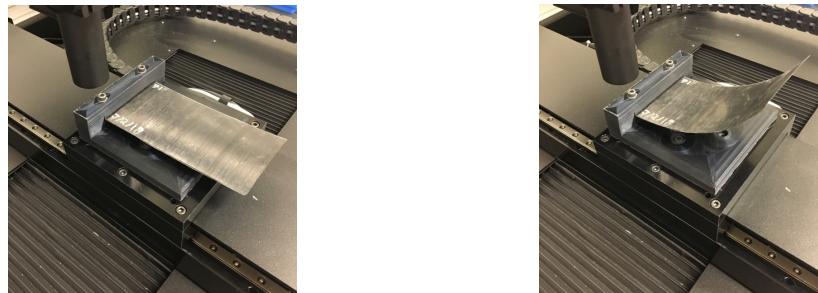
(a) laminate in the post cure shape clamped (b) laminate in the snap through shape clamped
