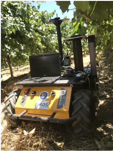
Fig. 1: The RAPID robot prototype, featuring a linear actuator mounted soil moisture probe and a data logger recording sampled values (visible on the right). This robot can collect soil moisture data while operating in the vineyard.
