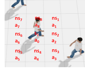
Fig. 1: Pedestrian motion model in a grid based workspace with adjoining states ns_1, ns_2, \dots, ns_8 and corresponding actions a_1, a_2, \dots, a_8 to reach those states.
