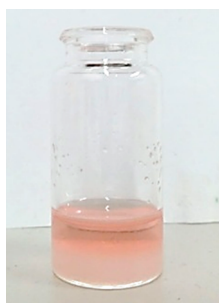
Figure 9. Solubility test for URCAT in bidistilled water.
