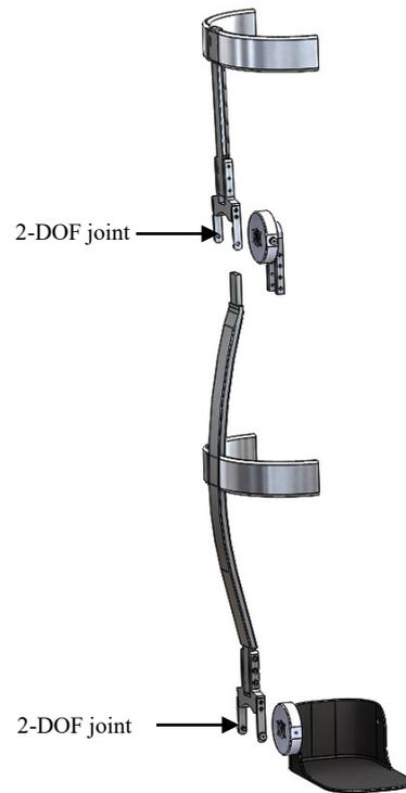
Fig. 1. Exploded view of 2-Degree-of-Freedom (DOF) joints of the Measurement exoskeleton system (developed for right leg)
