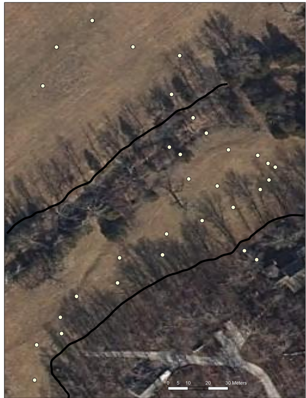
FIGURE 1. Locations of survey points in the test comparing Reach RS and Leica GS15. Each point was recorded by both instruments, and then the computed positions were compared. Note the placement of points in open spaces and near trees.
