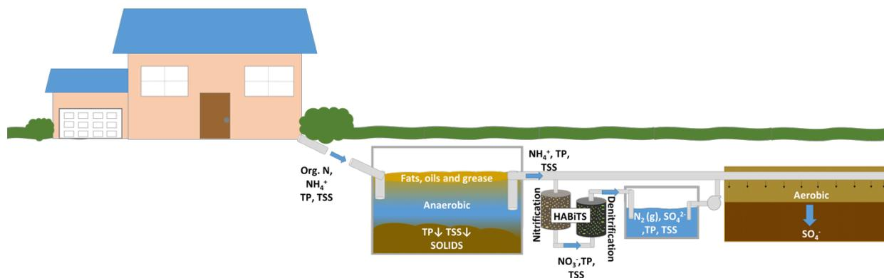
**Figure 1.** Hybrid Adsorption and Biological Treatment System (HABiTS), enhanced Onsite Wastewater Treatment Systems (OWTS)
