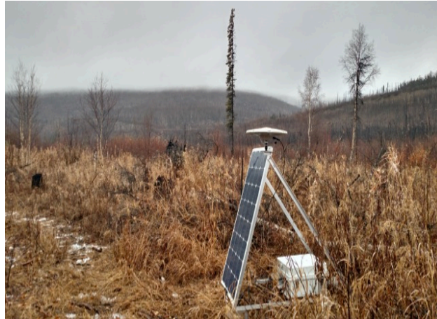
Figure 5. Example MAHALI box for GNSS deployment in challenging environments
