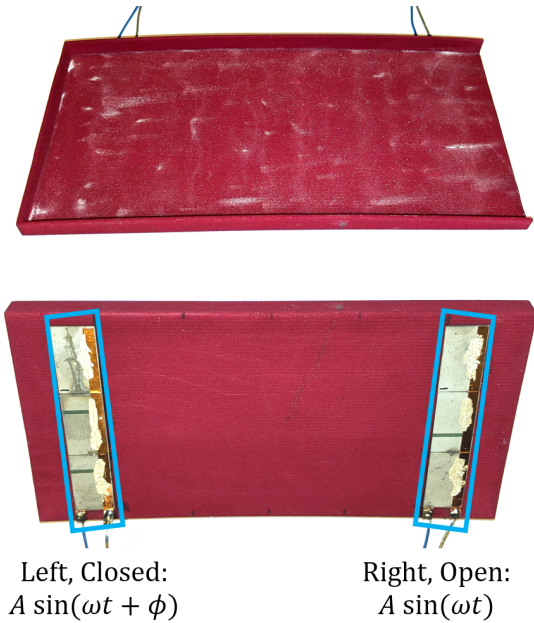
FIGURE 1. Images of the the top (upper) and bottom (lower) surfaces of the tray. Two rows of piezoelectric elements (PZTs) acting as actuators can be seen: the left group near the closed end of the tray and the right group near the open, lip-less end. Equations are representative of excitation signals to the two groups, where \phi is the phase difference applied to the left group.
