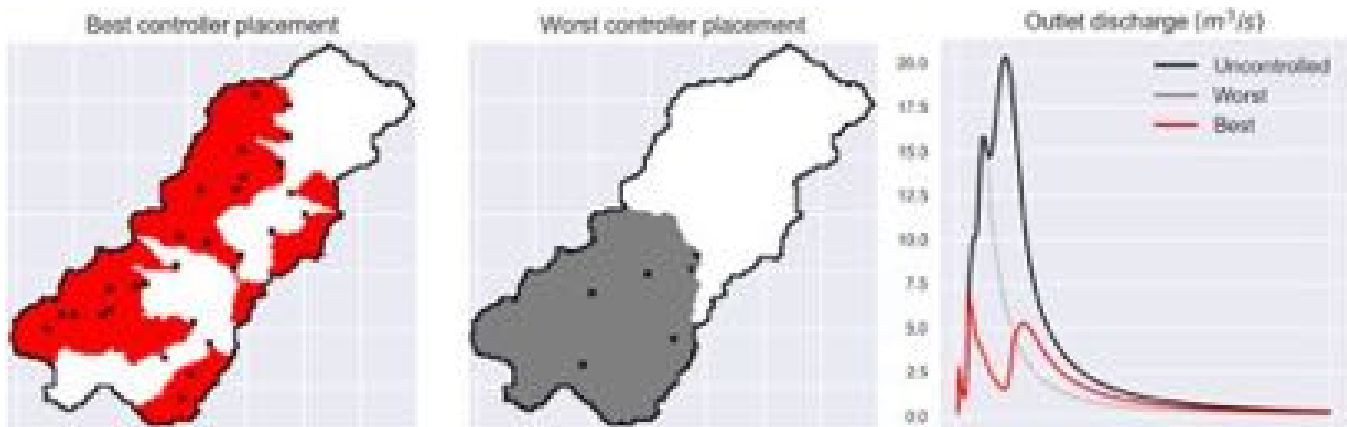
Fig. 7. Left: Best controller placement in terms of peak discharge ( k = 30 controllers, using the controller placement algorithm). Center: worst controller placement in terms of peak discharge ( k = 6 controllers, randomized). Controller locations are indicated by black crosses, and controlled partitions are indicated by colored regions. Right: hydrographs associated with the best and worst controller placement strategies (1-year storm event, volume capture scenario).
