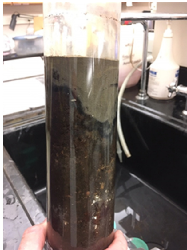
Fig. 3. Picture of a fringe core with a lighter mud layer on the top covering the darker, peat layer.
