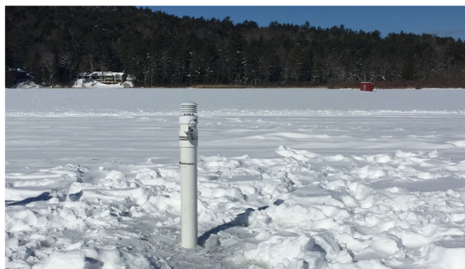
Fig. 4. The February deployment of the SIMB-3 prototype in a freshwater pond near Hanover, NH. The prototype deployment validated the SIMB3's ability to accomplish the operational and scientific design requirements.
