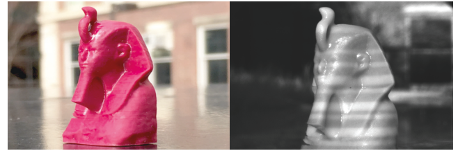
Fig. 16. NIR LayerCode tags in sunlight. The NIR LayerCode tags remain invisible in sunlight (left), but become visible when imaged with a NIR filter in front of the camera (right). No additional light source is needed.
