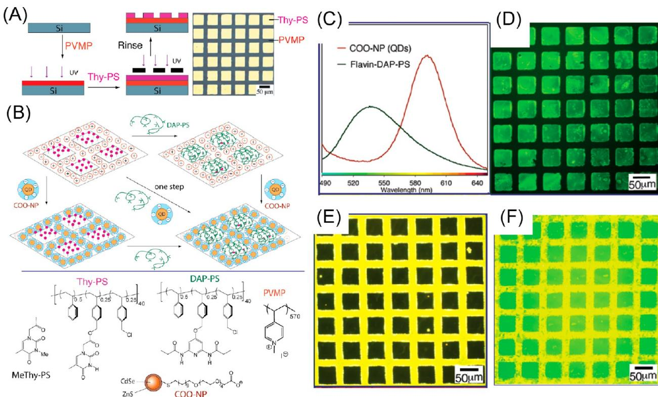
**Figure 7.** (A) Fabrication of a patterned PVMP/Thy-PS surface and its optical micrograph. (B) One-step sequential orthogonal functionalization process using DAP-PS and COO-NP and the chemical structures of the materials. (C) Fluorescence emission spectra of DAP-PS and COO-NP. Fluorescence microscopy of surfaces modified using (D) DAP-PS, (E) COO-NP, and (F) both components in a one-step process. Adapted with permission from ref 52. Copyright 2006, American Chemical Society.
