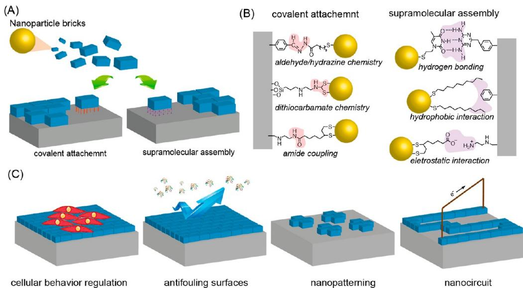
Figure 1. (A) Schematic illustration of NP-based nanobrick coating strategies. (B) Examples of NP coatings using covalent or supramolecular strategies. (C) Schematic illustration of NP-based coating applications.
