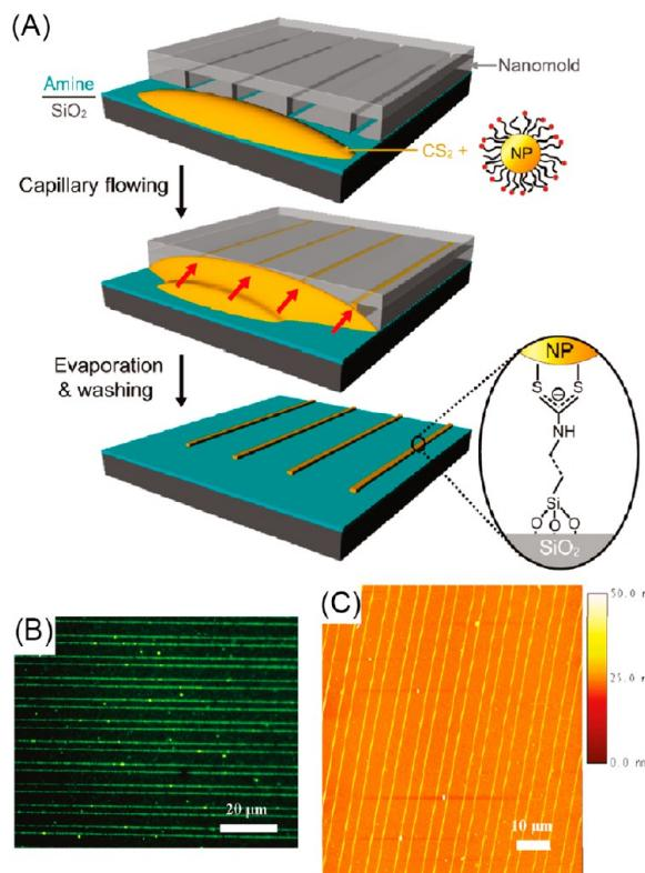
**Figure 6.** (A) Fabrication of 1D NP arrays using NAMIC coupled with DTC chemistry. (B) Fluorescent image of patterned QD-TOH NPs. (C) AFM topography image of patterned FePt-TOH NPs. Adapted with permission from ref 50. Copyright 2010, American Chemical Society.
