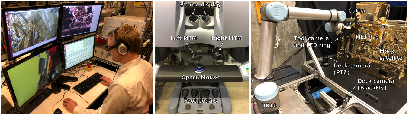
Fig. 1. Left: Conventional teleoperation keyboard and GUI (KB); Center: da Vinci master console (dV) with space mouse; Right: remote robot with satellite (see Fig. 2 for closeup of cutting assembly). Left image shows NASA operator performing trial with augmented virtuality (AV) visualization on 3D monitor (lower left monitor). Operator is wearing noise-canceling headphones and 3D shutter glasses. Conventional (CAM) visualization is similar, except that lower left monitor shows 2D camera image. Lower right monitor shows robot control GUI (also shown in Fig. 4).
