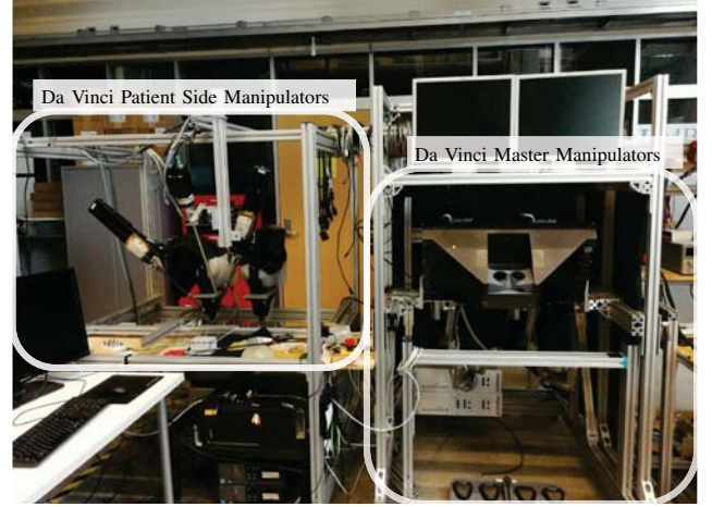
Fig. 1. The dVRK experimental setup. Two slave arms were commanded through two master arms.
