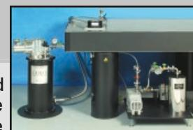
Existing LHe cooled cryostats and probe stations can be converted to cryogen-free operation with the addition of an external cryocooler, the Janis Recirculating Gas Cryocooler (RGC4). Instead of using LHe from a storage vessel, the RGC4 delivers a stream of 4K helium to the cryostat or probe station. Contact Janis today for more information.
