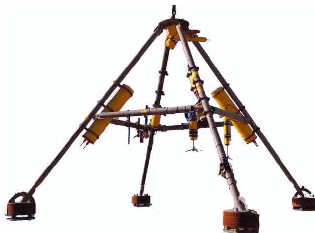
Figure 3. Underwater quadpod placed on the seabed off the SE corner of Martha's Vineyard. The quadpod is equipped with multiple acoustic and pressure sensors to measure the seabed and local hydrodynamics.
