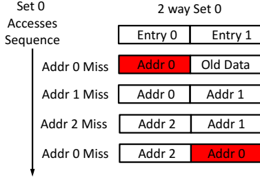
Figure 2: Examples of Reuse Distances(RD). The RD of Addr 0 is 3.
