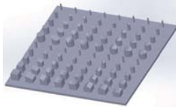
Figure 11. Diagram of 3D-printed circular and square targets in various areas and profiles.
