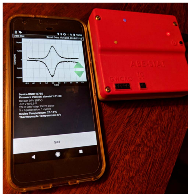
Figure 2. ABE-Stat (red enclosure at right) interfaced wirelessly to Android app on smartphone (Google Pixel 1 pictured).
