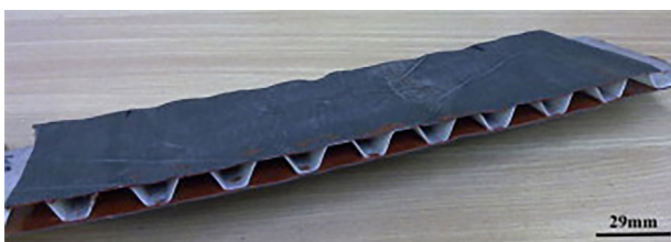
Figure 9. The coated corrugated core used in the airfoil morphing structure. [24] (Reproduced with permission. [24] Copyright 2013, Elsevier).
