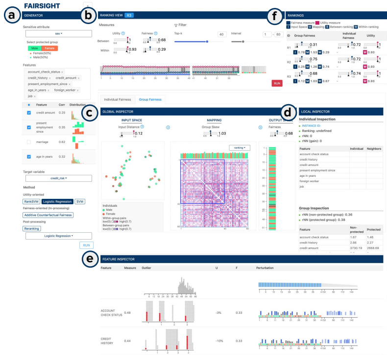
Fig. 2. The workflow of fair decision making in FairSight . (a) It starts with setting up inputs including the sensitive attribute and protected group. (b) After running a model, the ranking outcome and measures are represented in Ranking View. (c) Global Inspection View visualizes the two spaces and the mapping process of Individual and Group fairness provided in the separate tab. (d) When an individual is hovered, Local Inspection View provides the instance- and group-level exploration. (e) In Feature Inspection View, users can investigate the feature distortion and feature perturbation to identify features as the possible source of bias. (f) All generated ranking outcomes are listed and plotted in the Ranking List View.
