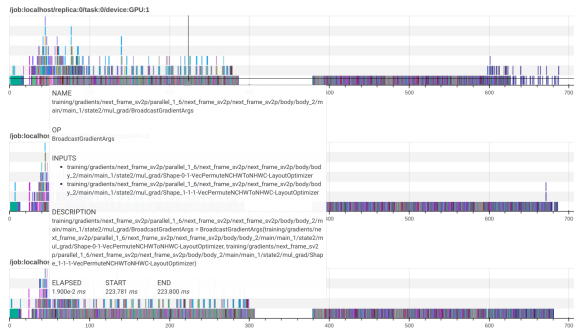
Figure 3: The timeline interface provides details of the execution of one iteration step. Each box represent an operation in the DataFlow DAG. There is a timeline for every resources on each machine. The trace is collected from next_frame_sv2p [4] model in tensor2tensor library [10].
