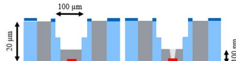
Fig. 6: Legend and orientation are the same as in Fig.4 (a) Result of Step 3 FIB opening and thinning to 100nm (b) Attack performed from Section II
