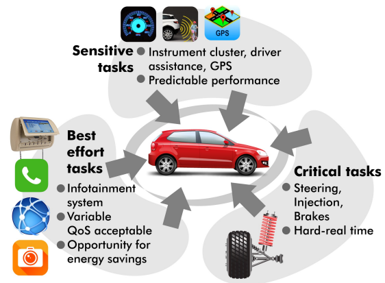
Figure 1: Envisioned MPSoC consolidation scenario.
