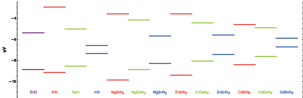
Figure 1. VBM and CBM levels with respect to vacuum level for ZnO and III-N and II-IV-N 2 compounds.
