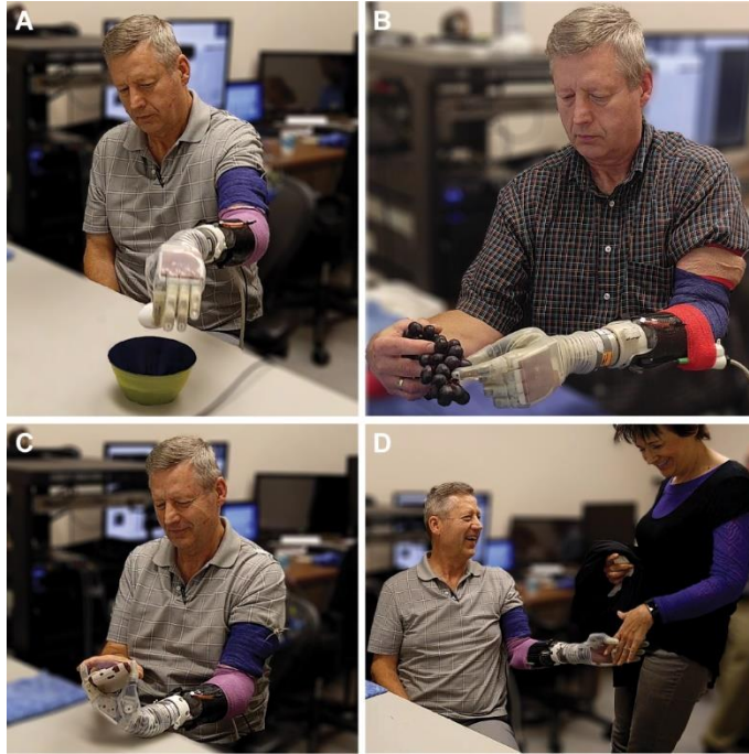
Fig. 6. Sensory feedback supports activities of daily living (ADLs). The participant performed several one- and two-handed ADLs while using the sensorized prosthesis, including: moving an egg (A) , picking grapes (B) , texting on his phone (C) , and shaking hands with his wife (D) .
