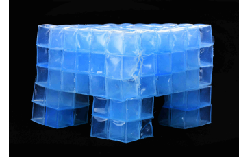
Fig. 2. The blue robot, made from thin-walled inflatable elastomer voxels.
