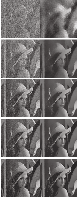
FIG. 2. Compressed sensing reconstruction of Lena using NLM-AMP, at undersampling ratio m/n = 0.5 : iterates \mathbf{x}^t + \mathbf{A}^T \mathbf{r}^t (left column) and \mathbf{x}^{t+1} = \eta_t(\mathbf{x}^t + \mathbf{A}^T \mathbf{r}^t) (right column) for t \in \{0, 1, 2, 3, 4\} . (Details in the main text.)
