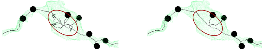
Fig. 3. Loop Removal. Since the thinning step preserves topology, any holes in the input segmentation cause loops in the skeleton. On the left, we see an example skeleton after thinning with several loops (the black spheres represent synapses). After refinement, these loops disappear, leaving a cleaner skeleton (right).
