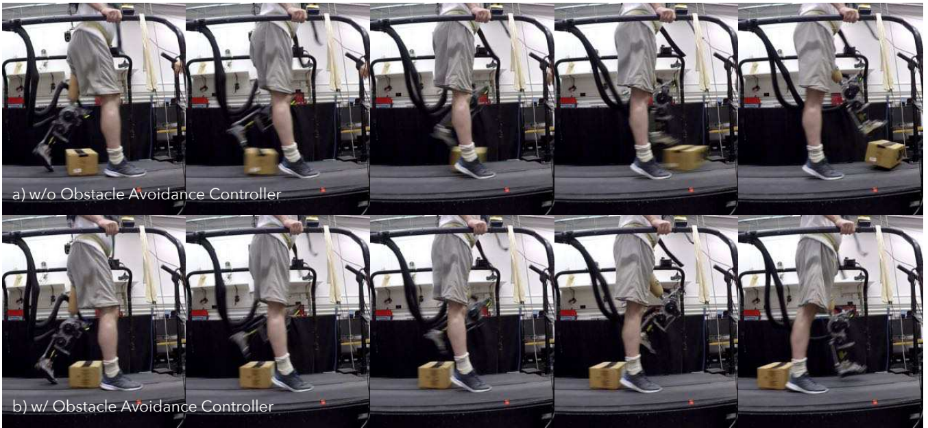
Fig. 1. a) Utilizing minimum jerk trajectories during swing does not allow for appropriate adaptation of swing trajectories to enable obstacle avoidance. b) Our adaptive system learns online to detect the presence of an obstacle from the amputee’s late stance/early swing movements. Once detected, the controller modifies the trajectories of the knee and ankle to achieve improved obstacle clearance.
