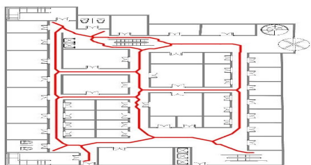
Figure 4: Final connectivity graph constructed by IBeaconMap.
